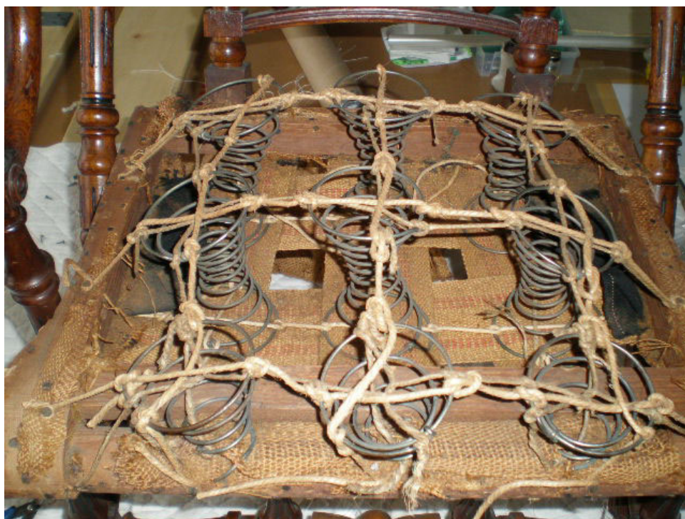
Fig. 4 The springs and lashing cords found within the chair's seat.
