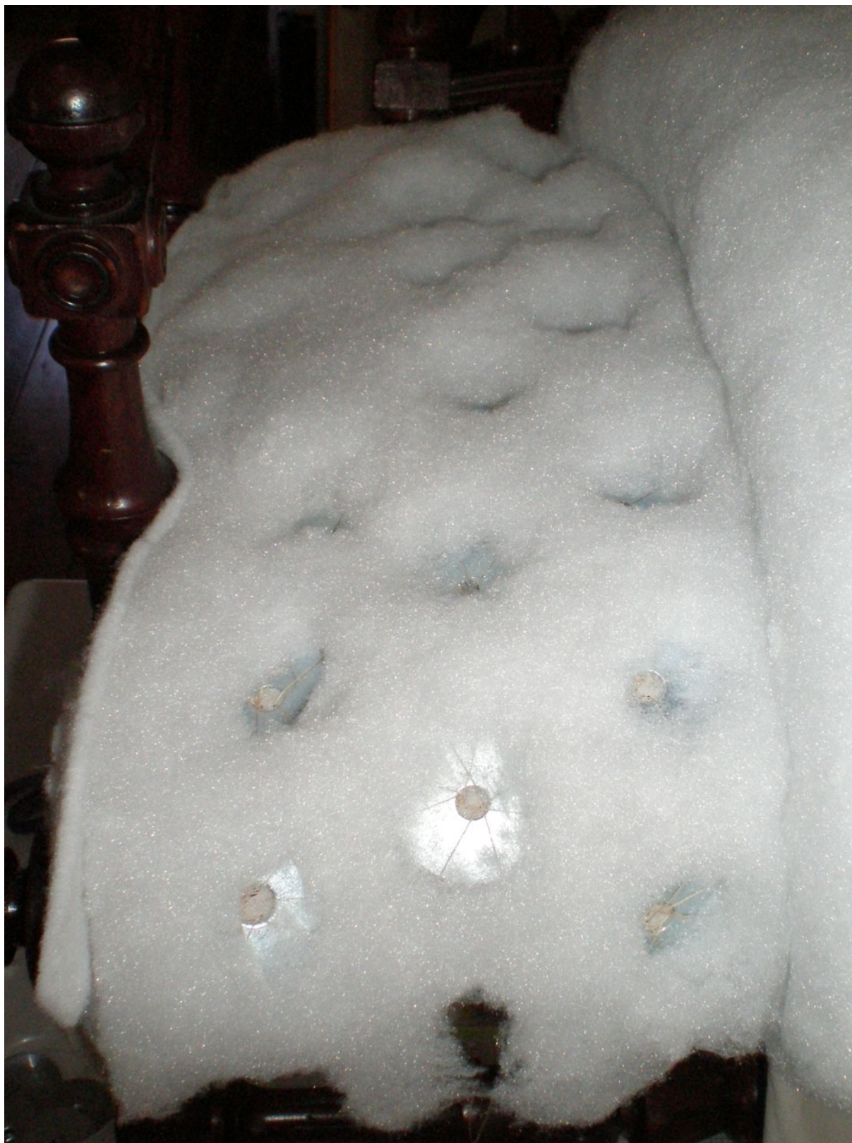
Fig. 7 Batting layers applied with cutout holes for deep tufting to be inserted and secured with the covered magnets.
