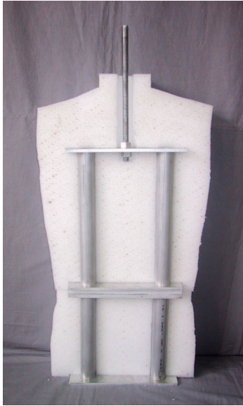
Figure 3a (left): Internal Armature embedded into the Ethafoam plank; Figure 3b (right): An elongated torso with stop-clamp access cavity.
