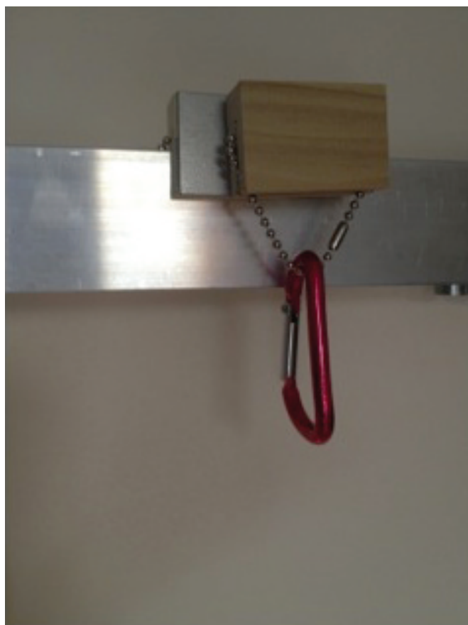
Figure 4: Wooden blocks with secured magnets or ferromagnetic materials made to rest on the upper edge of the aluminum bar and support a weighting bucket.
