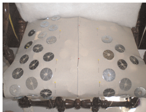
FIG. 8. Batting layers applied on top of the spring cover cloth with stitched washers. The batting is cut away from the metal washers to reduce bulk and thus the gap between the magnet and the washer.
