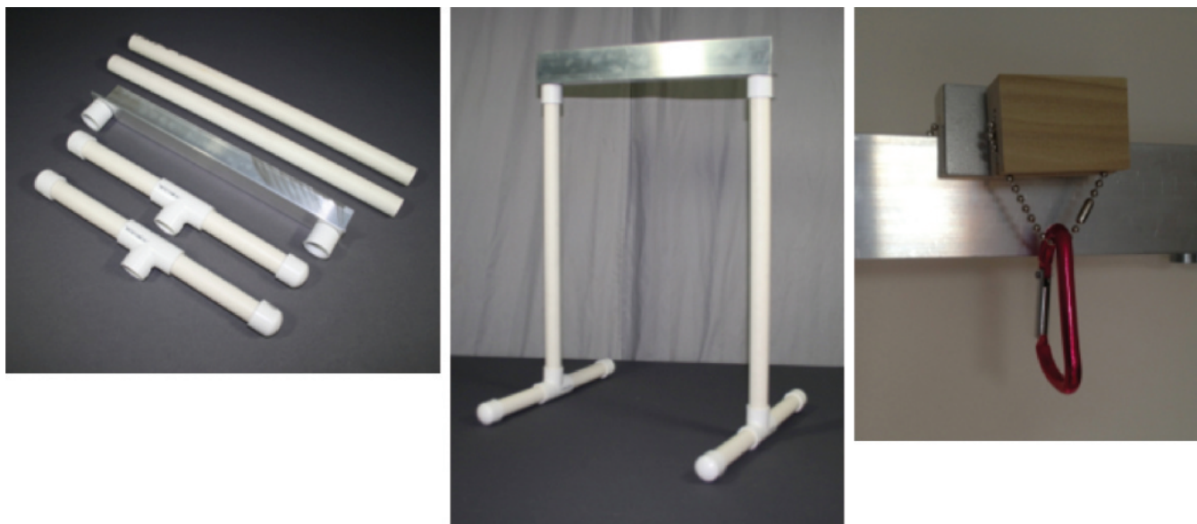
Figure 3: The jig is made of 3/4" PVC pipe for the legs, and an upper horizontal aluminum "L" piece. Wooden blocks with secured magnets, or ferromagnetic materials, are made to rest on the upper edge of the aluminum bar and support a weighting bucket (Woods, 2013; Spicer, 2014).
